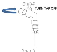
2.6 Remove the hose plug/connector from the tap
