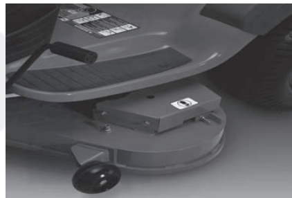
Fabricated Deck Shell Example Below
